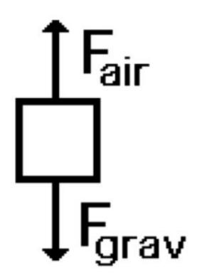
Gravity pulls down on the skydiver while air resistance pushes against gravity.
